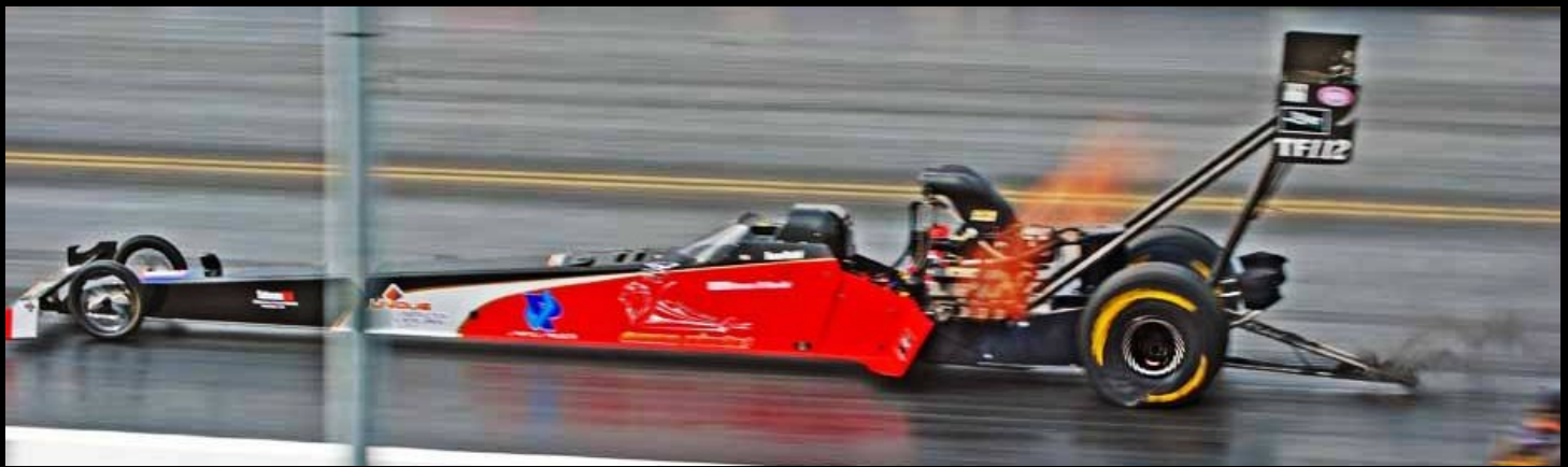
This could be when the Maltese Lion's car began to lose a three-second ET, the tyre starting to bulge as it went into shake mode – but Duncan drove it hard to a 4.02 at 303mph, yet another consistent pass for his Rune Fjeld Motorsports car. Meanwhile severe shake, pedallin' and smokin' the tyres eventually activated Urs' safety cut-out and deployed his chutes, the car cruising through the traps to a 6.12 at 131.38 with chutes flapping in the breeze
