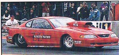
PRO 10 - Arto Sandberg, Finland (EF20/21G) Ford Mustang '95 - 7.26/305kmh Chassis: Jerry Haas Engine: Ford Wedge 500 by Q-mile Engineering
